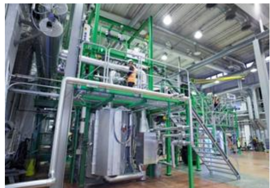
Fig. 4. Chemical looping combustion pilot scale test facility of VTT, located in Espoo, Finland. (Credit: VTT)
